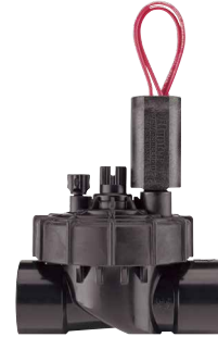
PGV-101JT-G Inlet Diameter: 1" Height: 5½" Length: 4½" Width: 3¼"
