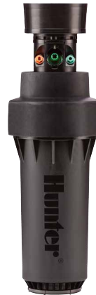
I80-00-SS Riser Mount I80-00-SS-ON Riser Mount Overall height: 9¾" Exposed diameter: 2¼" Inlet size: 1½"
